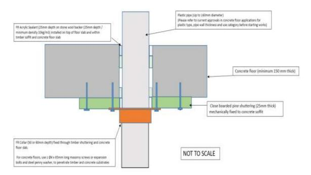
In our opinion, the fire test carried out with the CLT floor is a more onerous case than the one described above and we feel comfortable that Protecta FR Collars will provide a fire resistance of El 120 with the shown minimum floor build up with plastic pipe (up to 160mm) already approved in concrete floor uses in terms of types, pipe wall thickness and defined pipe usage.
