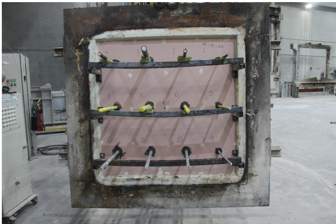
Figure 2 – Exposed face prior to test commencement
