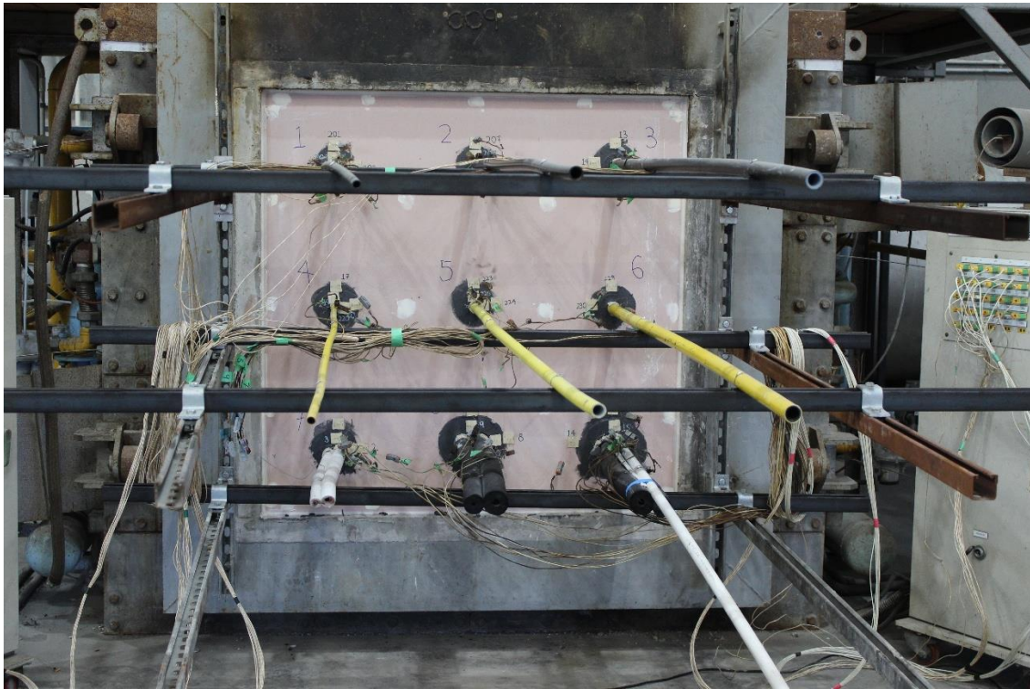
Figure 1 - Unexposed face prior to test commencement
