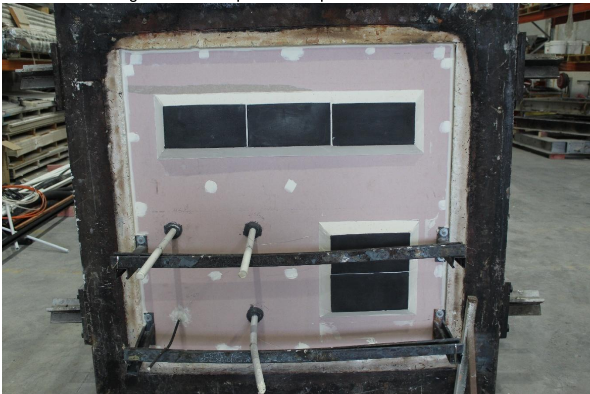
Figure 2 - Exposed face prior to test commencement
