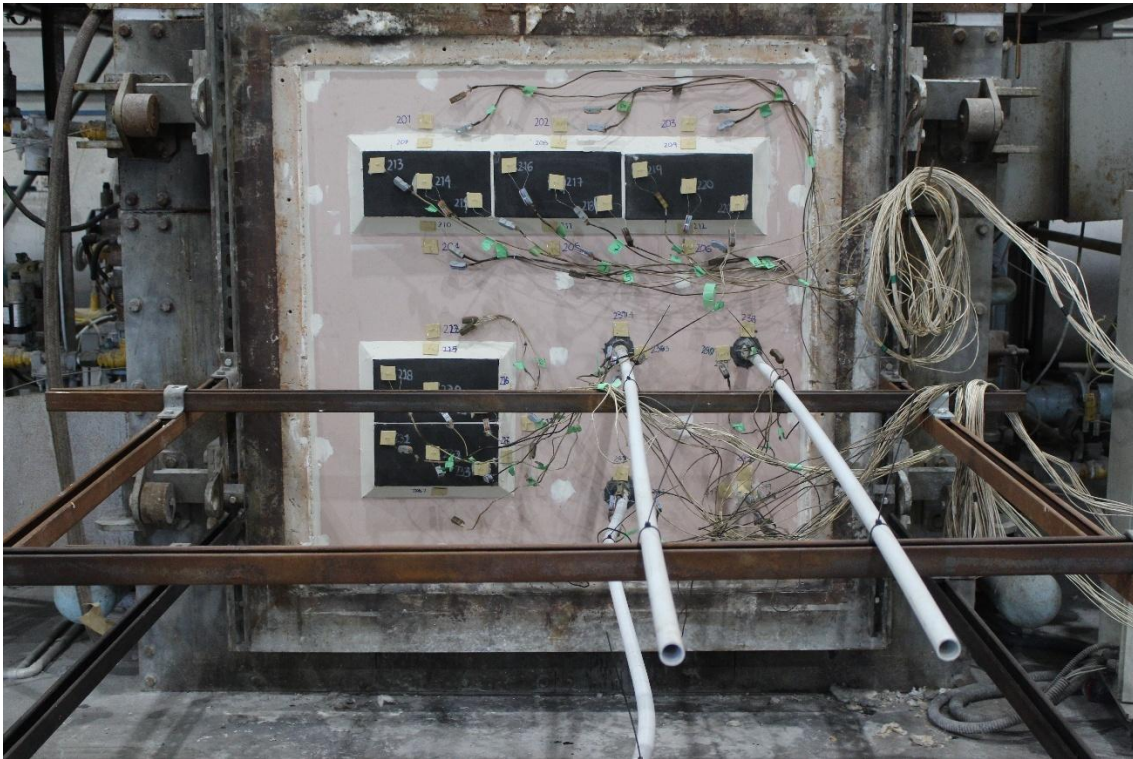
Figure 1 - Unexposed face prior to test commencement
