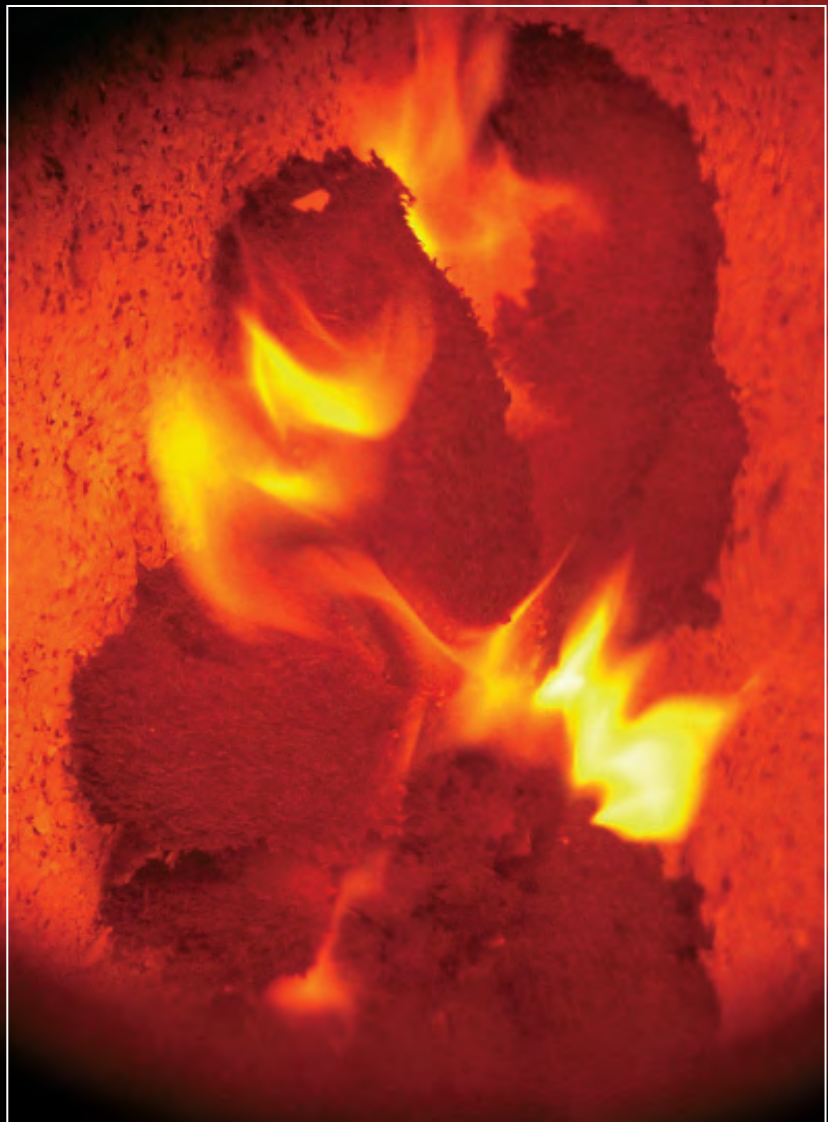
Activated Allproof Intumescent during fire testing in a plasterboard wall.
